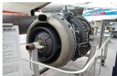
YS-11 Engine Rolls-Royce RB.53 Dart Mk.543-10 Provided by Tokorozawa Aviation Museum [Before 1970s]
